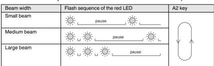
Hold down the A1 key for 2 seconds to save the selected beam shape, terminate the parameterisation and ensure that the sensor returns to normal mode. Briefly press the A1 key to return to Step 1 (parameterisation of the output function).
